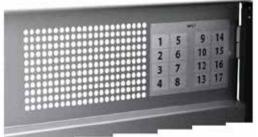
You install an input module by sliding the module into a module slot in the input section of the headend unit and push it till the module clicks into place.
